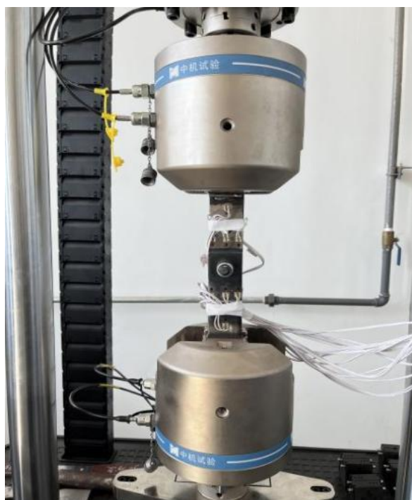
Figure 2. The strength test of riveted joints
